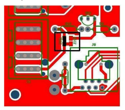
Make a jumper on JIS1 and cut the JIS2 jumper (see black box in the image)
