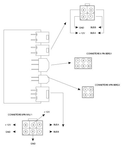
Figure 12 "Layout of Node Connectors"
