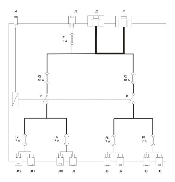
Figure 11 "Power Hub logic diagram"
