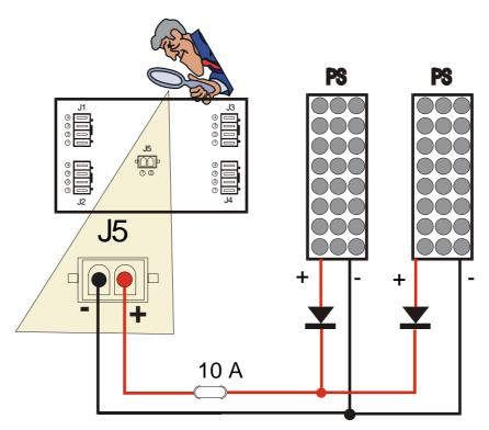
Figure 5 "Assembly of double Panel"
