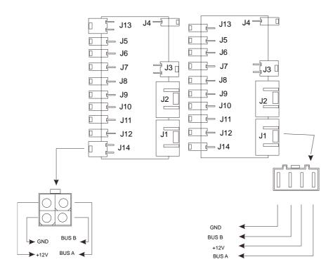
Figure 10 "Layout of Floor and Ceiling Power Hub connectors"
